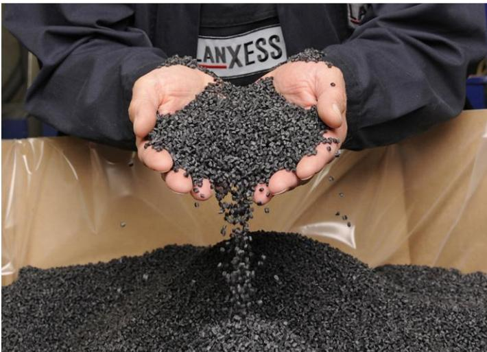
Durethan and Pocan engineering plastics (PA 6, PA 6.6 and PBT compounds) are used in numerous applications, above all in the automotive industry plus the electrical/electronics sector, but also in the construction industry, in medicine and in sports and leisure products. Photo: LANXESS AG
